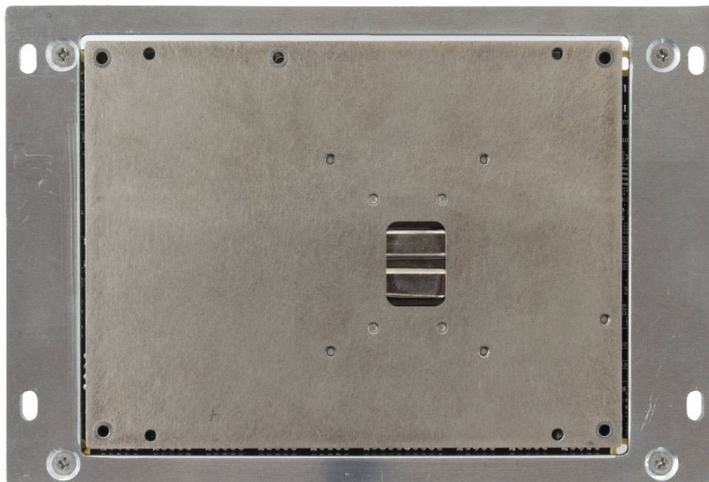
Bottom view showing Basic size COM + heat spreader nested in mounting plate
